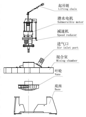
are compact and uniform, Due to the negative caused by the impeller in high speed movement status strengthened the self-suction function, the dynamic efficiency of the equipment is improved.
